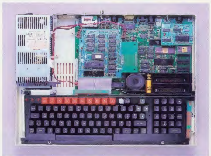
Turbo exposed: co-processor board with 65C102 to left and Econet top right
